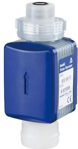
The EFS Flow meter mounts directly onto most EWN-Y pumps models directly below the manual air vent valve. It is available in a PVDF body with options of Titanium or Hastelloy C pin materials and FKM or EPDM seal materials at the connections. The EFS Flow meter can only be connected directly to an EWN-Y pump at this time.
